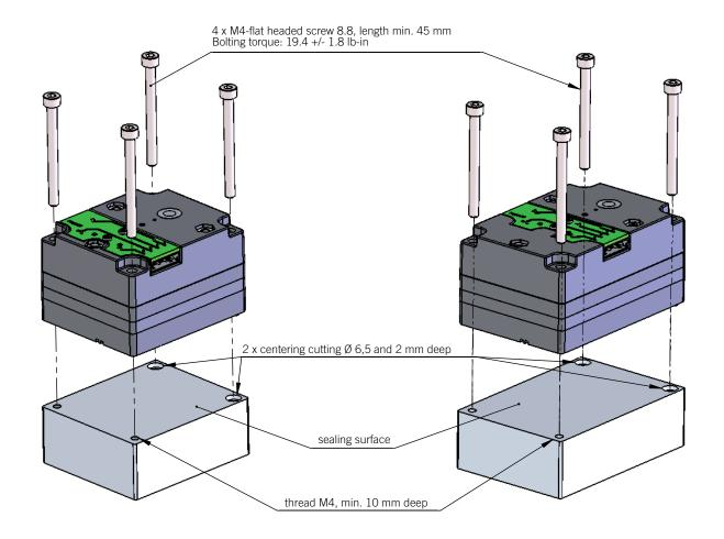
Specifications to sealing surface:  $\boxed{\bigcirc}$  0,05  $\boxed{\bigcirc}$   $\boxed{Ra 1,6}$
